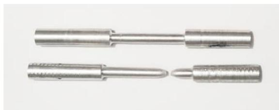
Fig. 3. Tensile test specimen
